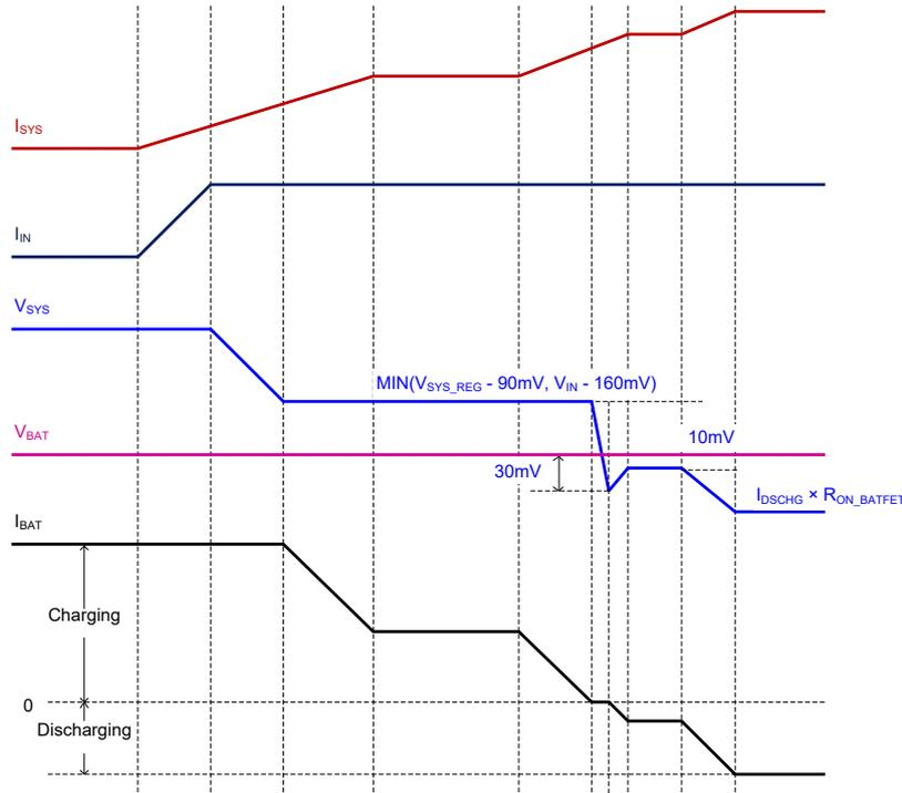
**Figure 6. Dynamic Power Management and Battery Supplement Operation Profile**
