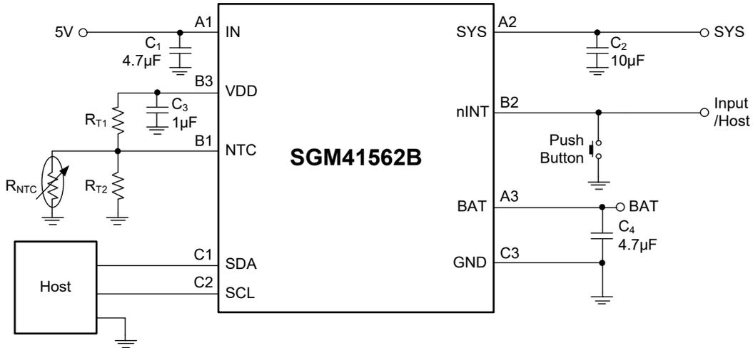
**Figure 13. SGM41562B Typical Application Circuit with 5V Input**
