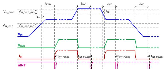
**Figure 4. Input Power Detection and nINT Signaling Timings**
