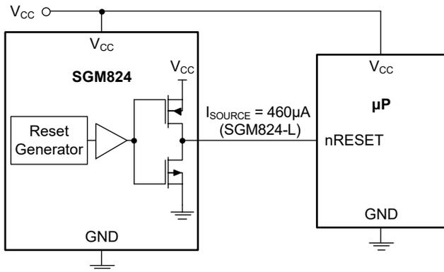
Figure 3. Interfacing to µP with Bidirectional Resets
