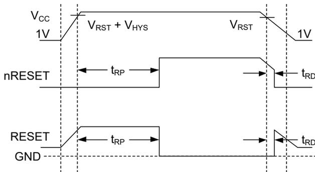
Figure 1. Reset Timing Diagram
