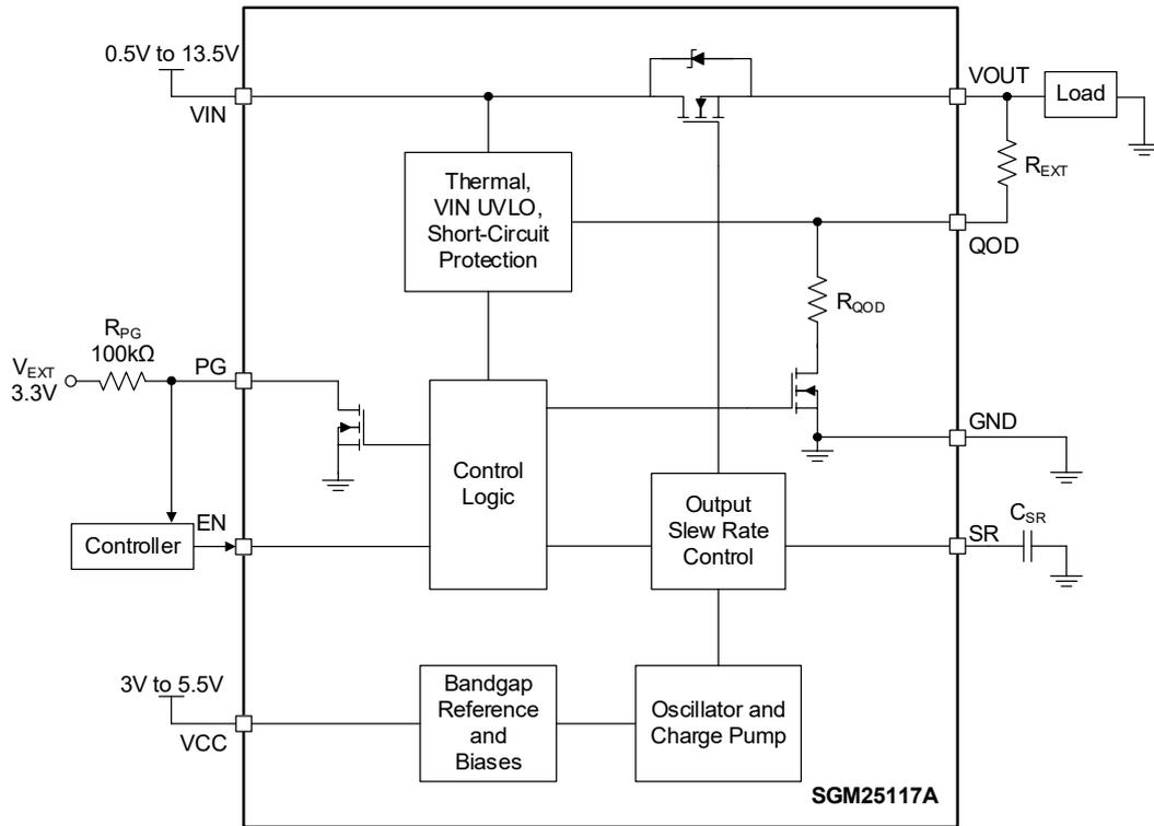
Figure 4. Load Switch
