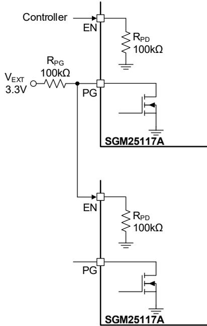
Figure 6. Power Sequencing with PG Output
