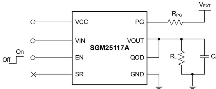
Figure 2. Test Circuit
