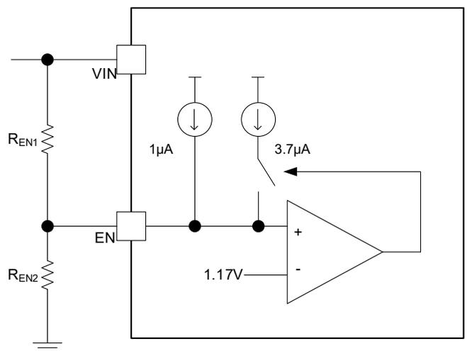
**Figure 3. V<sub>IN</sub> UVLO Adjustment Circuit**
