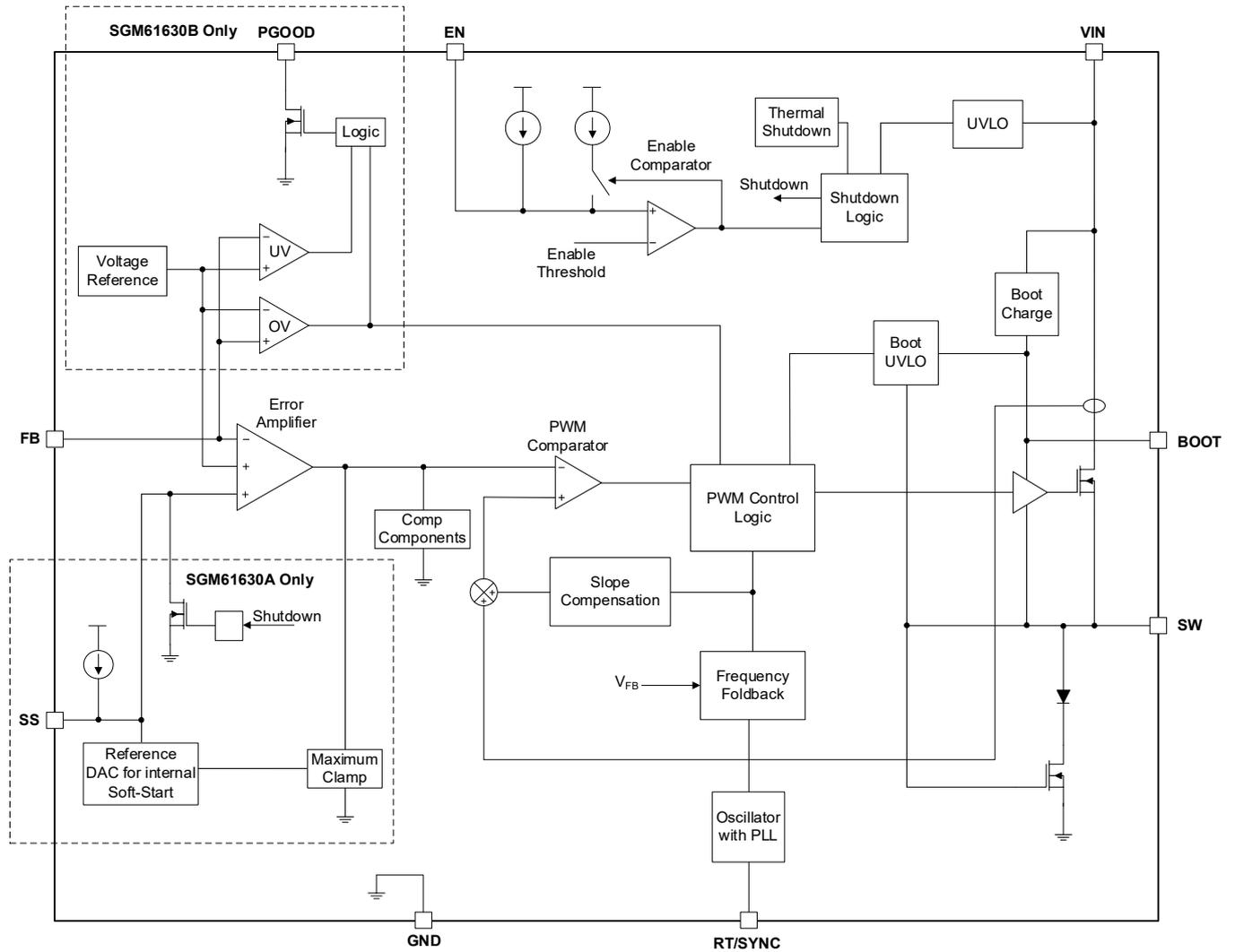
NOTE: SS pin is for the SGM61630A version and PGOOD pin is for the SGM61630B version.
