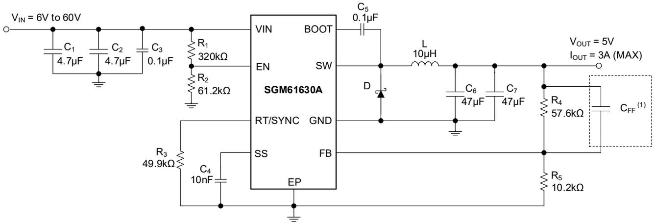
NOTE: 1. In low input voltage condition, C<sub>FF</sub> = 33pF is recommended.
