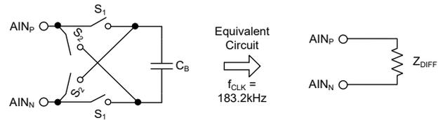
**Figure 5. Simplified Analog Input Circuit**
