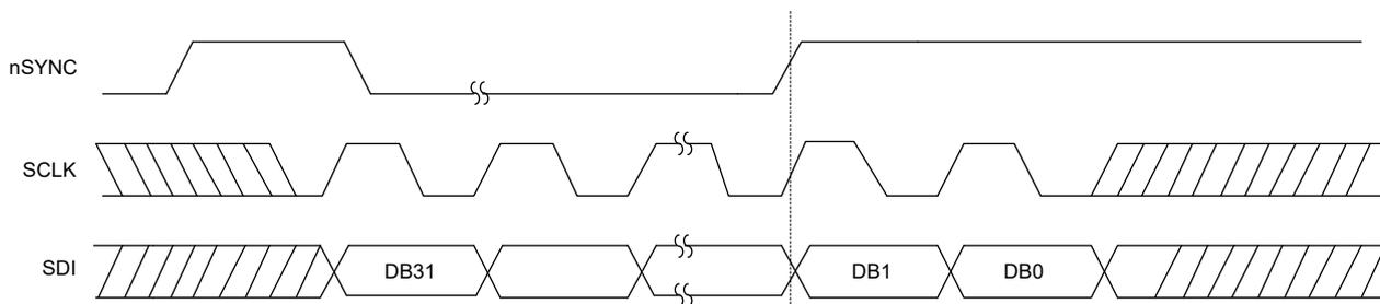
**Figure 5. nSYNC Invalid Interrupt timing**
