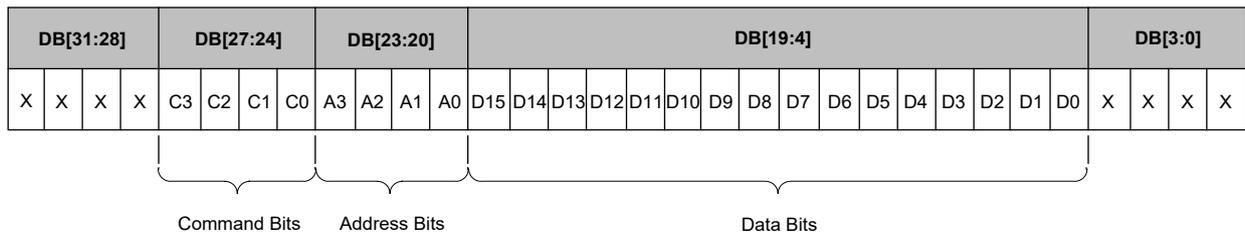
**Figure 4. SGM5349-16 Input Register Contents for DAC output**
