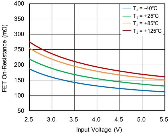
Low-side FET R<sub>DS(on)</sub> vs. Input Voltage
