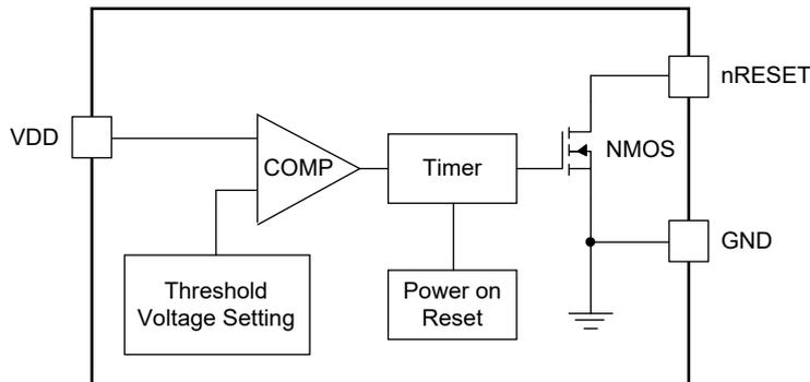
Figure 3. Block Diagram
