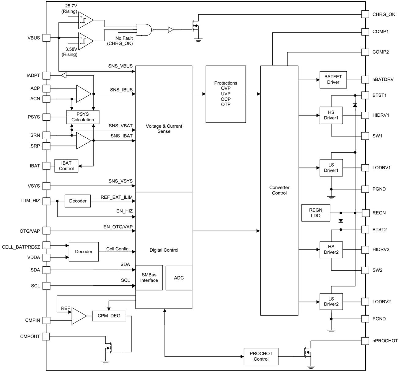
Figure 3. Block Diagram
