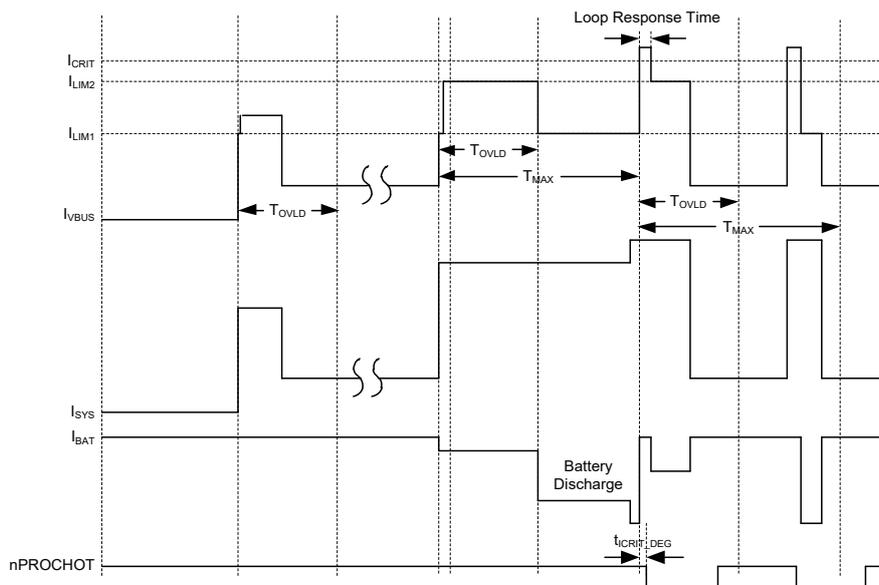
Figure 4. Two-Level Adapter Current Limit Timing Diagram
