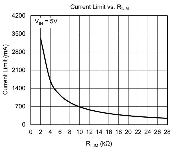
**Figure 6. Current Limit Threshold ( $I_{ILIM}$ ) vs. Current Limit Programming Resistor ( $R_{ILIM}$ )**
