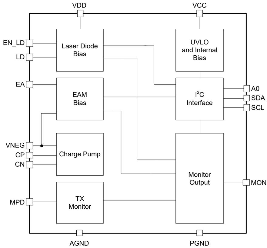
Figure 3. Block Diagram
