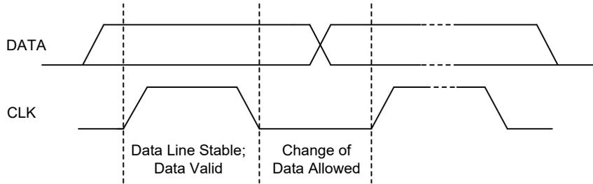
Figure 7. Bit Transfer on the Serial Interface
