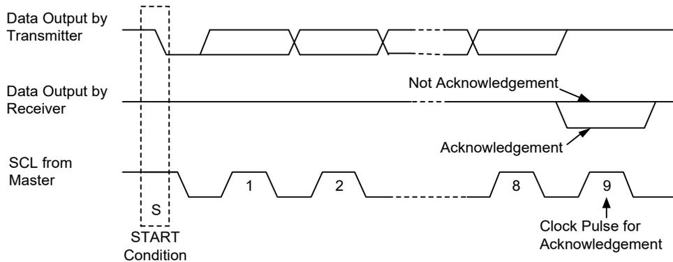
Figure 8. Acknowledgement on the I<sup>2</sup>C Bus
