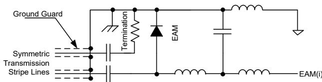
**Figure 5. Typical Application Circuit of EAM Bias**
