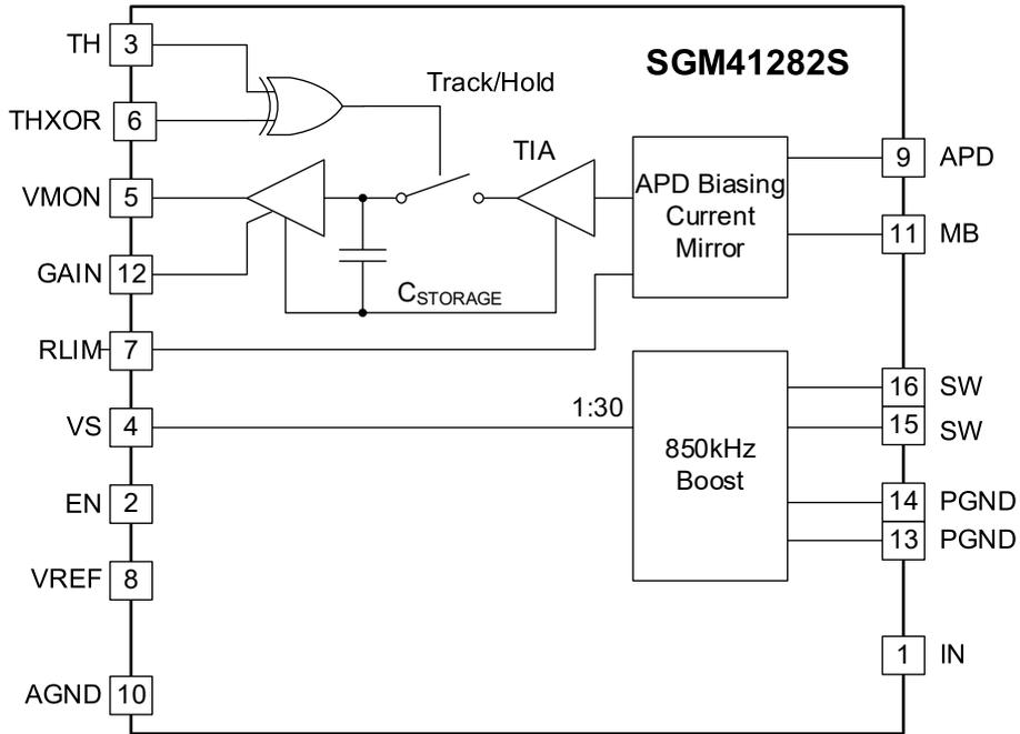
Figure 2. Block Diagram
