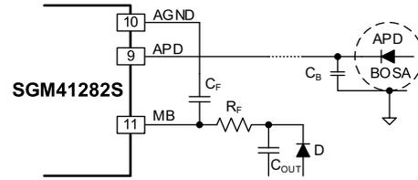
**Figure 4. An RC Filtering for Ripple Suppression**
