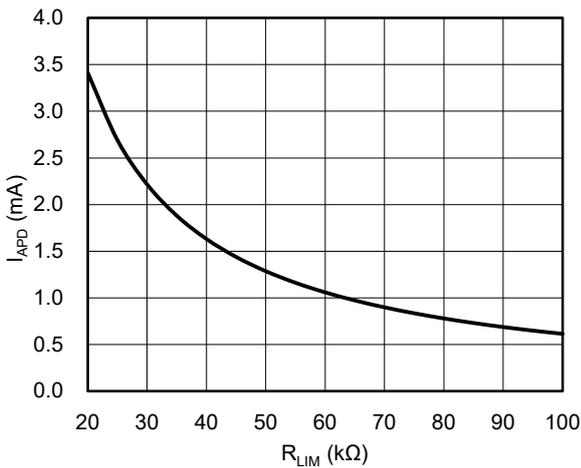
**Figure 3. APD Current Limit vs. R<sub>LIM</sub>**
