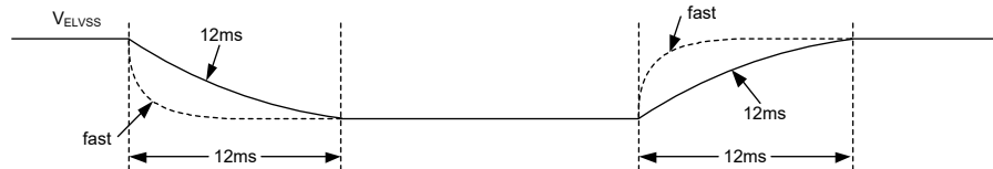
Figure 3. V_{ELVSS} Transition Time Control
