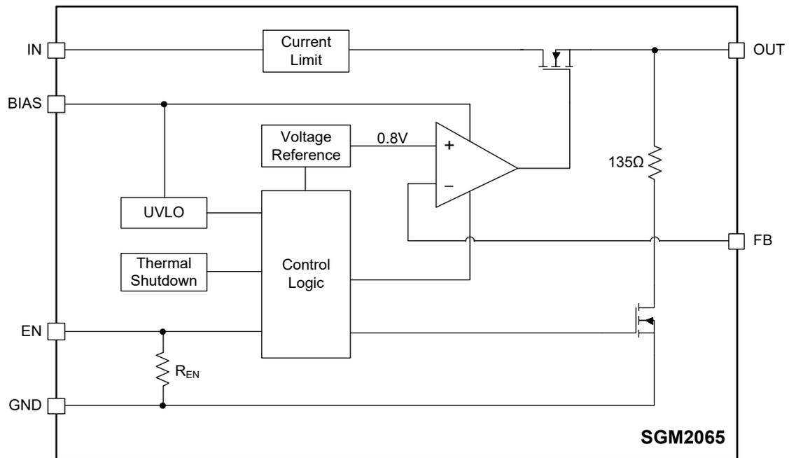
Figure 2. Block Diagram
