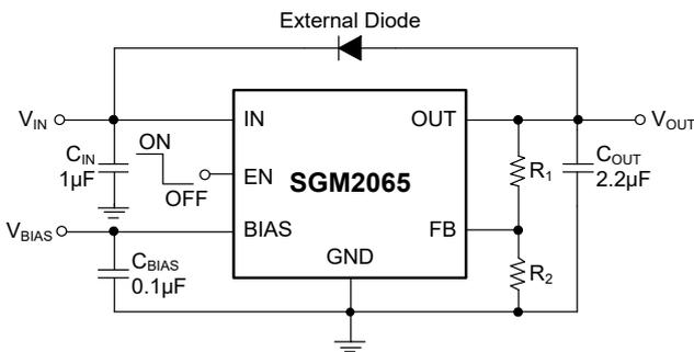
Figure 4. Reverse Protection Reference Design
