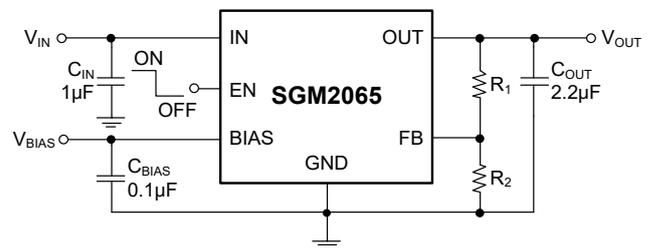
Figure 3. Adjustable Output Voltage Application
