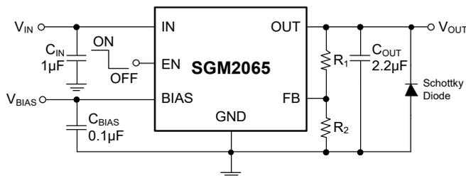
Figure 5. Negatively Biased Output Application
