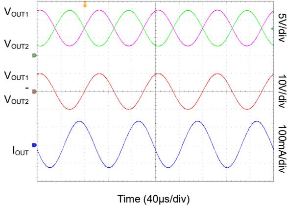
**Figure 5. Actual Output Waveform from Resolver Excitation Circuit (+V<sub>S</sub> = 15V, -V<sub>S</sub> = 0V, f = 10kHz)**
