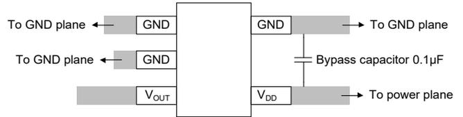
**Figure 4. Recommended Layout of SC70-5 Package**
