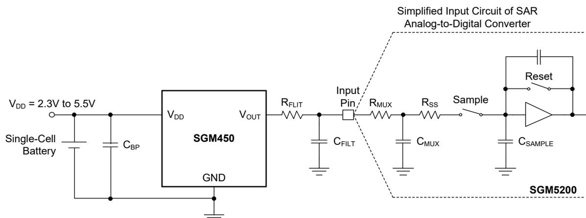
Figure 2. Recommended Connections to an ADC Input Stage
