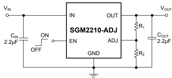
$$V_{OUT} = V_{ADJ} \cdot (1 + R_1/R_2)$$
