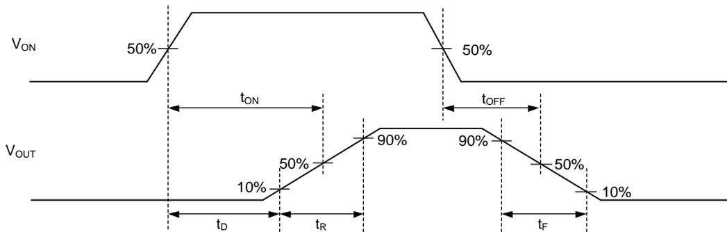
Figure 3. Turn-On and Turn-Off Waveforms
