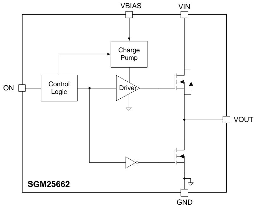
Figure 4. Block Diagram
