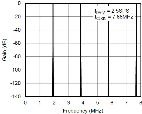
Figure 11. Frequency Response Out to 7.68MHz
