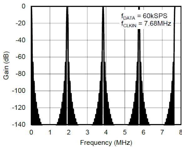
Figure 10. Frequency Response Out to 7.68MHz
