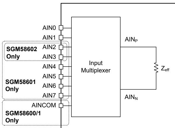
**Figure 6. Analog Input Effective Impedances with Buffer On/Off**
