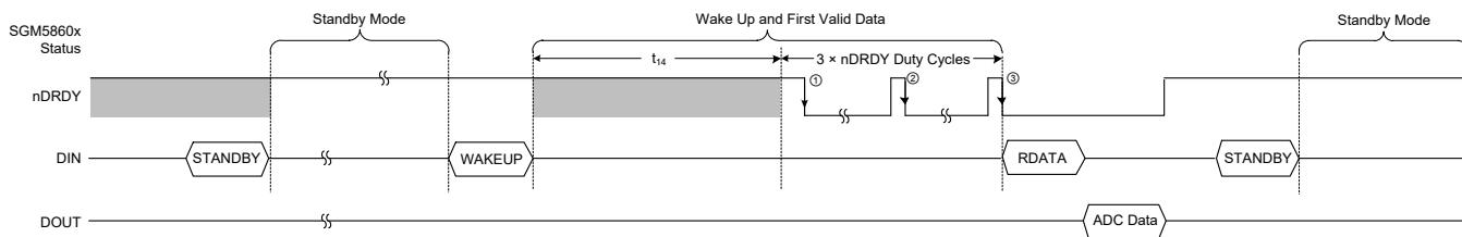
**Figure 13. One-Shot Conversions Using the STANDBY Command**
