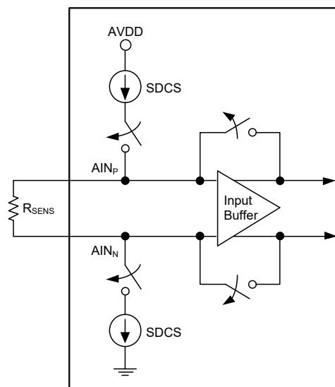
**Figure 5. Sensor Detection Circuitry**
