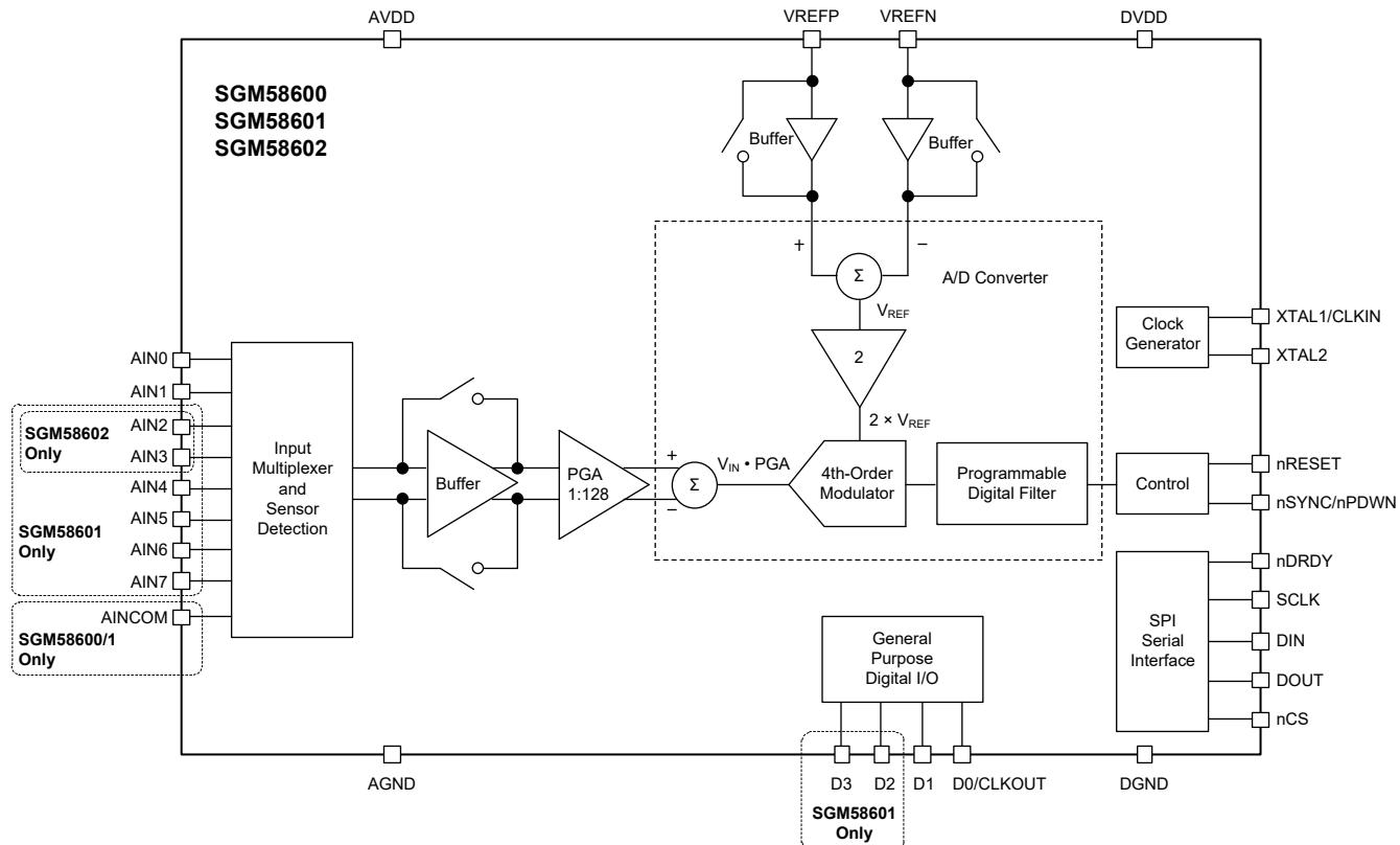
**Figure 4. Block Diagram**
