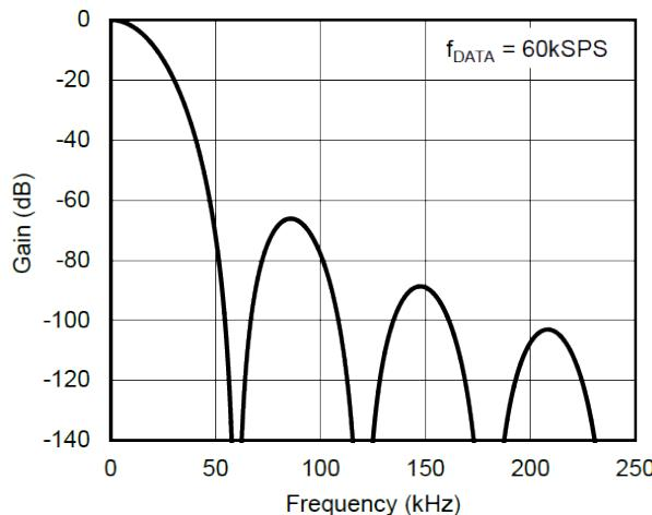
Figure 8. Frequency Response (Data Rate = 60kSPS)
