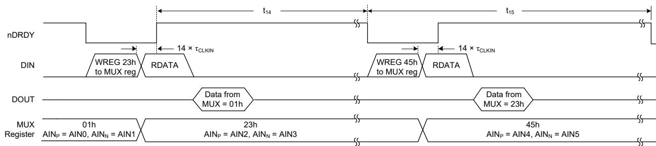
**Figure 12. Cycling the SGM5860x Input Multiplexer**
