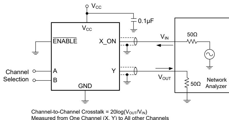
**Test Circuit 7. Channel-to-Channel Crosstalk**
