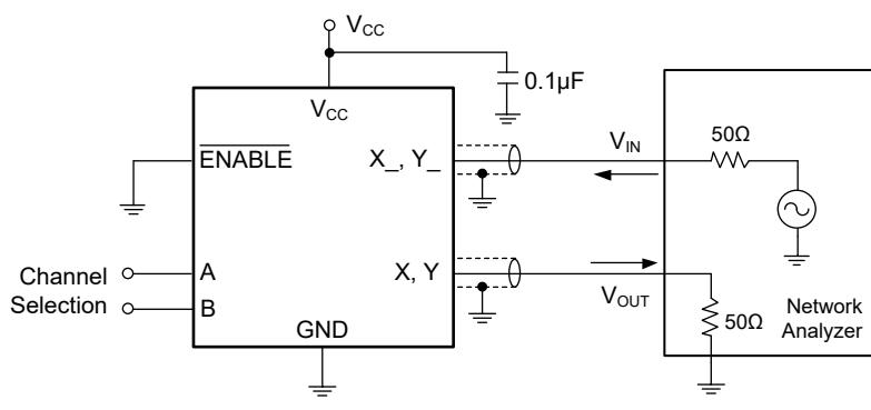
Test Circuit 6. On Loss
