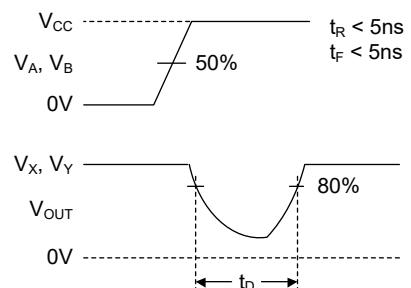
Test Circuit 3. Break-Before-Make Delay Time ( $t_D$ )
