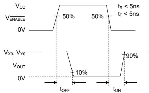
Test Circuit 2. Switching Times ( $t_{ON}$ ,  $t_{OFF}$ )
