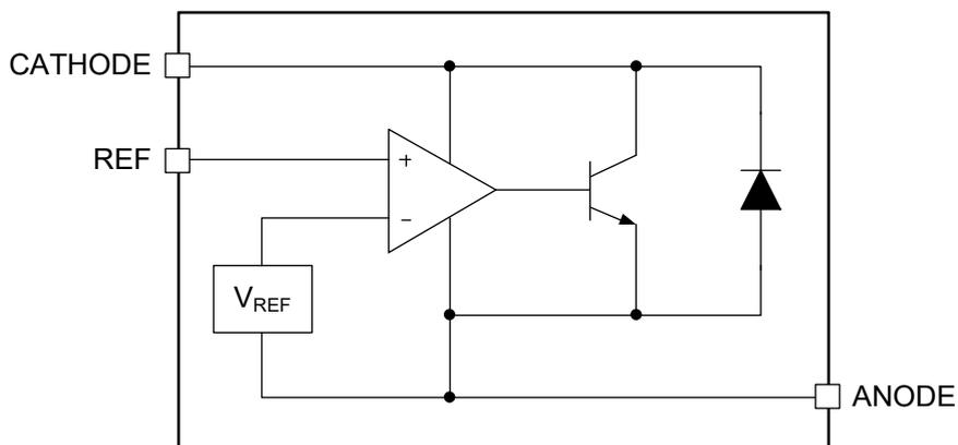
Figure 2. Equivalent Diagram
