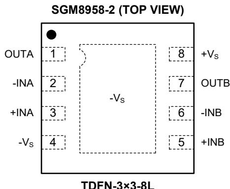
NOTE: For TDFN-3x3-8L package, exposed pad can be connected to  $-V_S$  or left floating.
