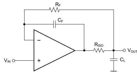
Figure 3. Circuit to Drive Heavy Capacitive Load
