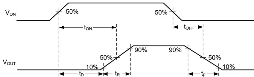
Figure 3. Timing Waveforms
