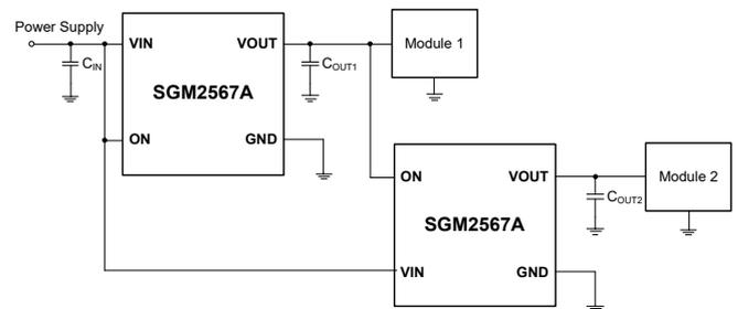
Figure 7. Power Supply Sequencing without a GPIO Input
