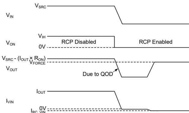
NOTES:  $V_{SRC}$  is the input power supply to the equipment.  $V_{FORCE}$  is the external power source forced at VOUT pin.  $I_{VIN}$  is the current of VIN pin.  $I_{OUT}$  is output load current.
