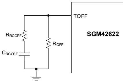
Figure 6. Programming PWM Off-Time
