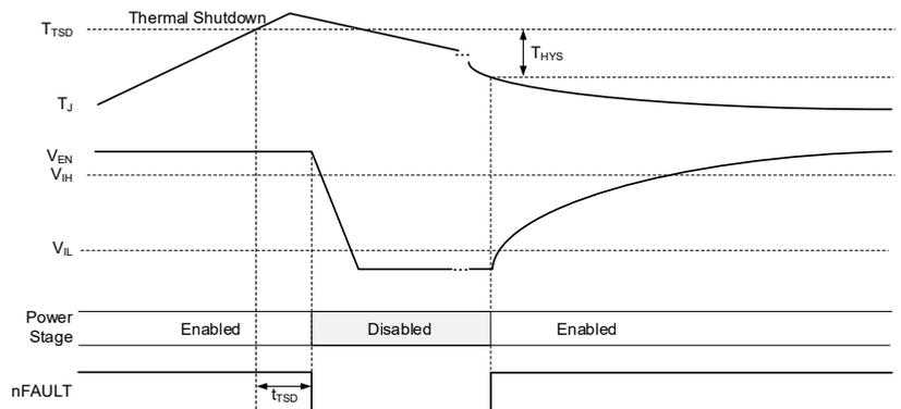
Figure 7. Thermal Shutdown in SGM42622
