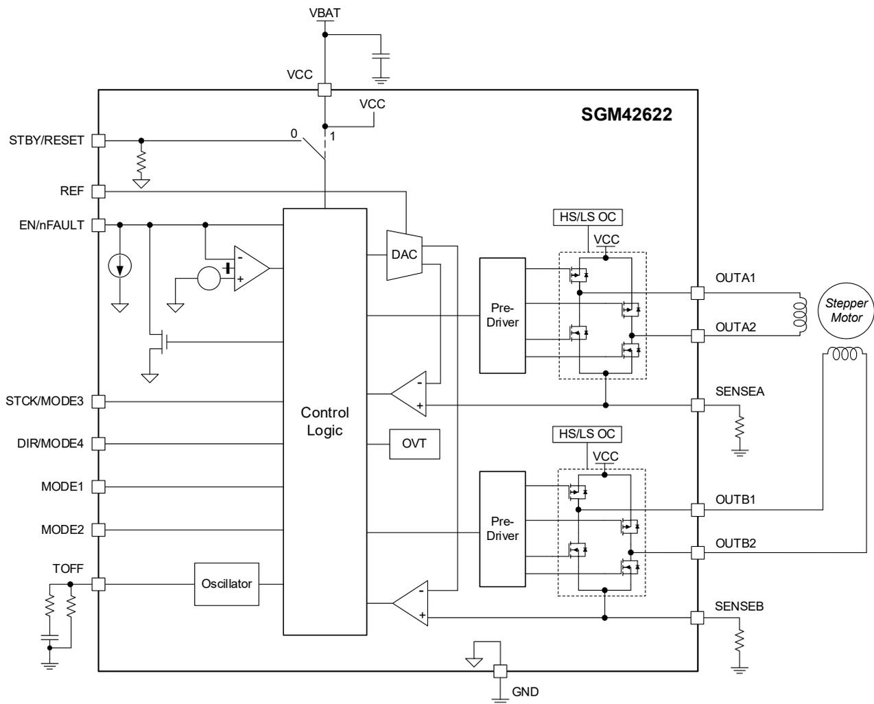
Figure 3. Block Diagram
