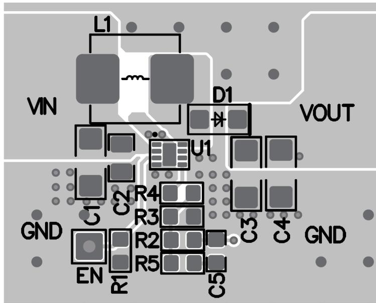
Figure 6. PCB Layout
