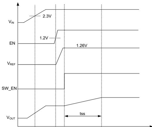
Figure 3. Typical Start-up Waveform
