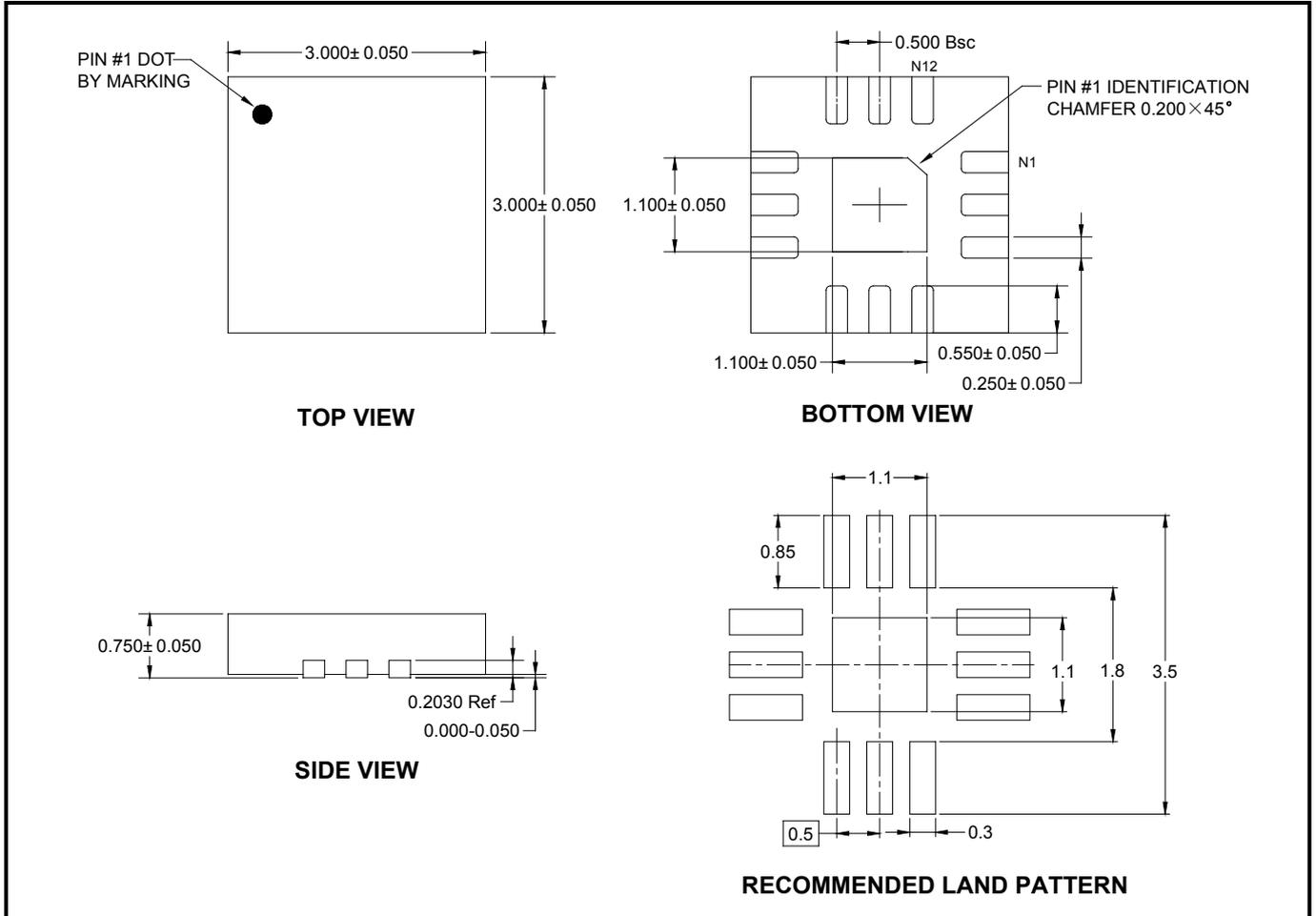
NOTE: All linear dimensions are in millimeters.
