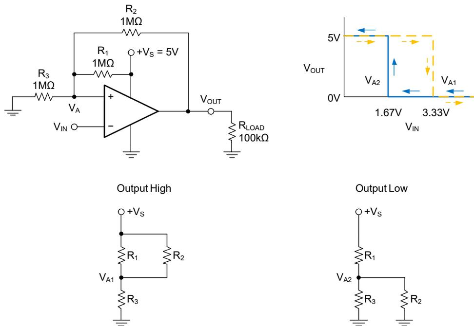
**Figure 3. SGM8714A-1 in an Inverting Configuration with Hysteresis**
