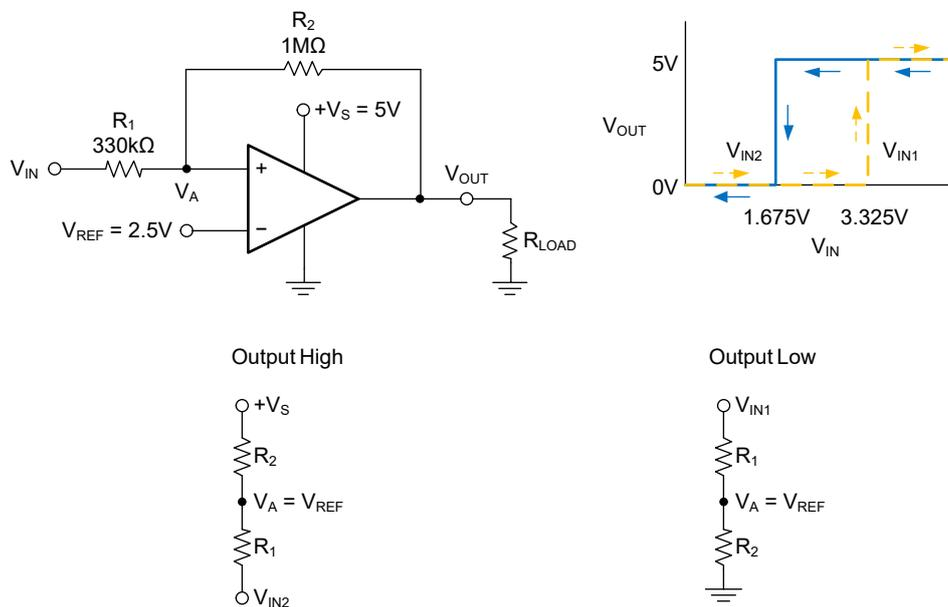
**Figure 4. SGM8714A-1 in a Non-Inverting Configuration with Hysteresis**
