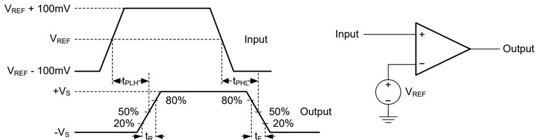
NOTE: The offset voltage and the hysteresis result in the propagation delay of the comparator output.
