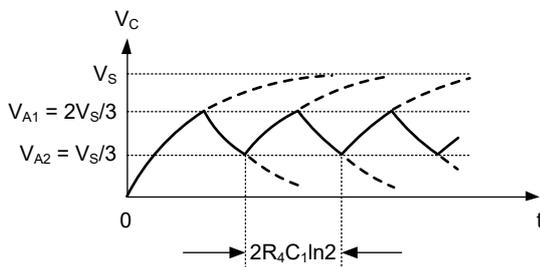
**Figure 8. Square-Wave Oscillator Timing and Thresholds**
