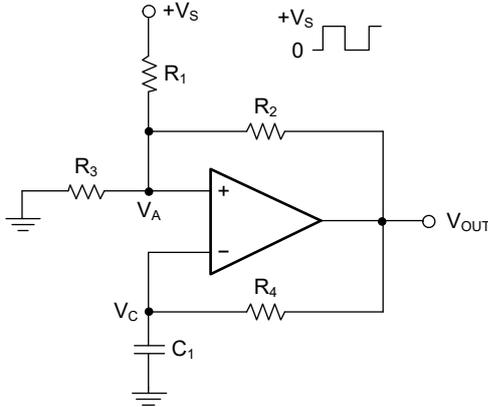
**Figure 7. Square-Wave Oscillator**
