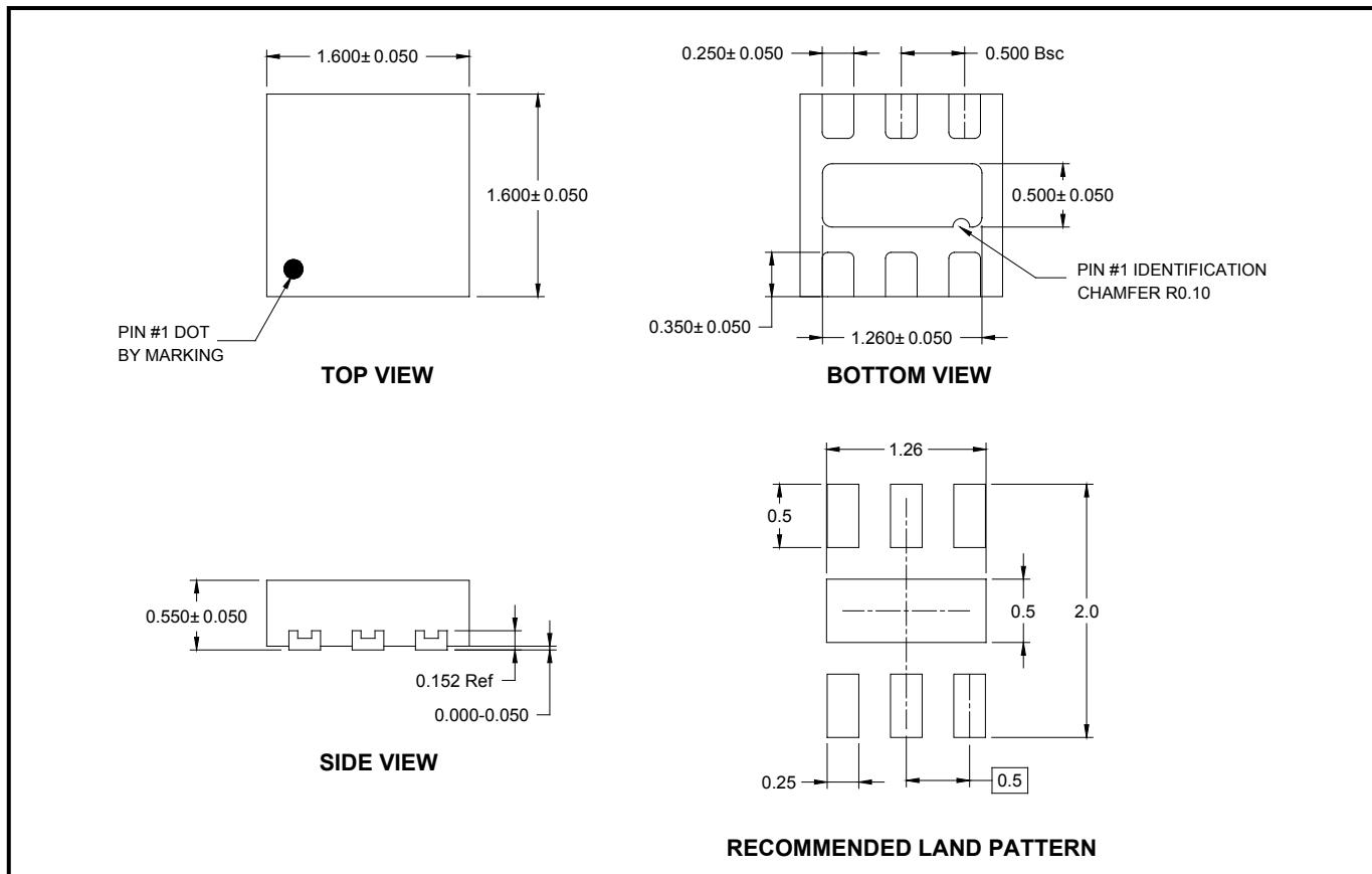
NOTE: All linear dimensions are in millimeters.
