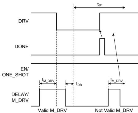
Figure 8. Manual MOSFET Power-On in One-Shot Mode
