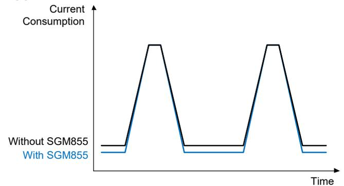
Figure 13. Effect of SGM855 on Current Consumption
