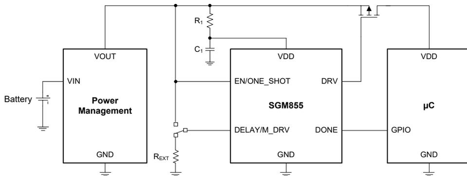
Figure 10. Manual MOSFET Power-On with SPDT Switch
