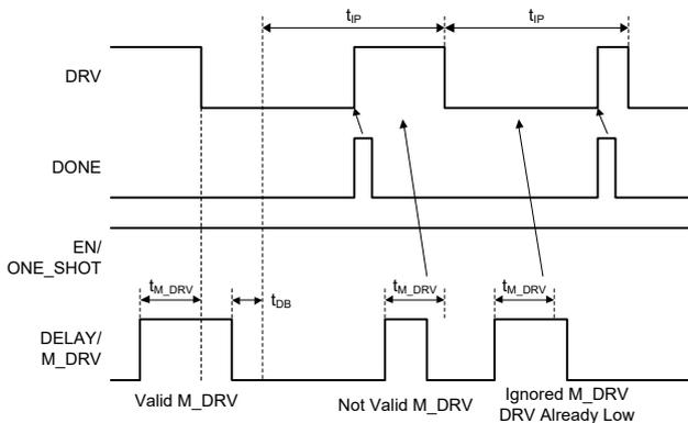
Figure 7. Manual MOSFET Power-On in Timer Mode
