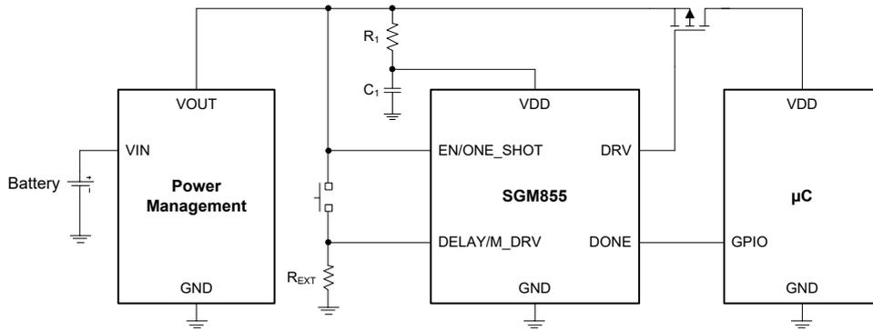
Figure 9. Manual MOSFET Power-On with SPST Switch
