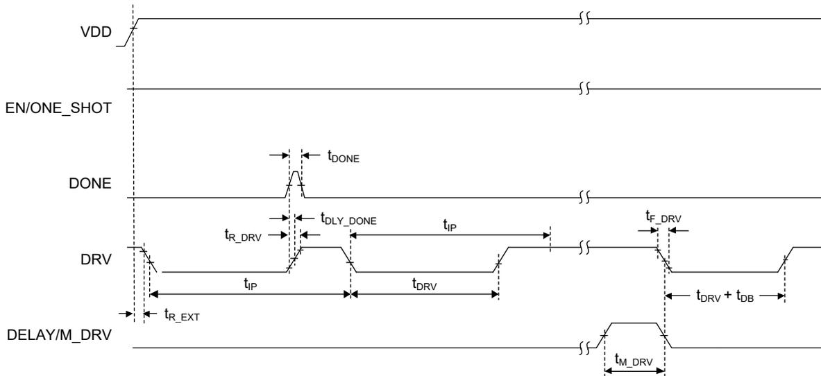
NOTE: It is recommended that the DONE signal must be given at least 200ns after the DRV falling edge to ensure the chip can correctly identify the DONE signal.
