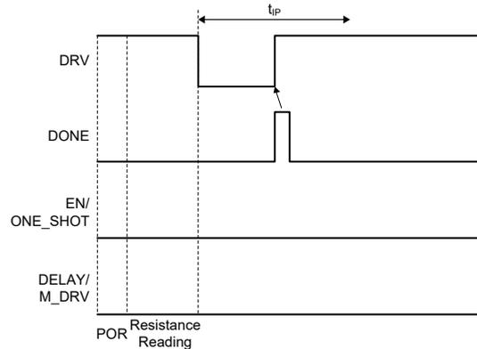
Figure 5. Startup One-Shot Mode (DONE Received within  $t_{IP}$ )
