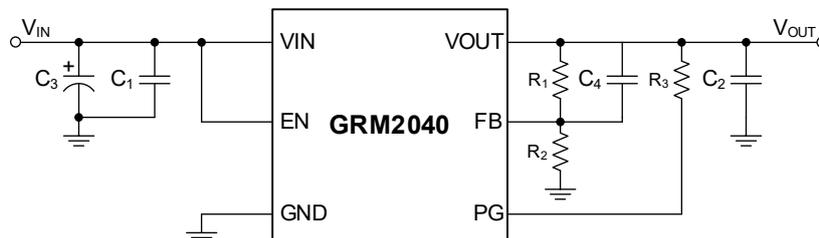
Figure 3. Application Circuit
