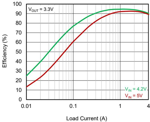
Efficiency vs. Load Current and Temperature
