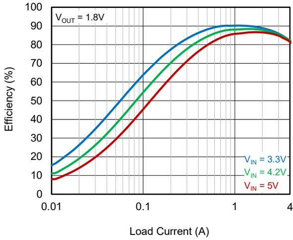
Efficiency vs. Load Current and Temperature
