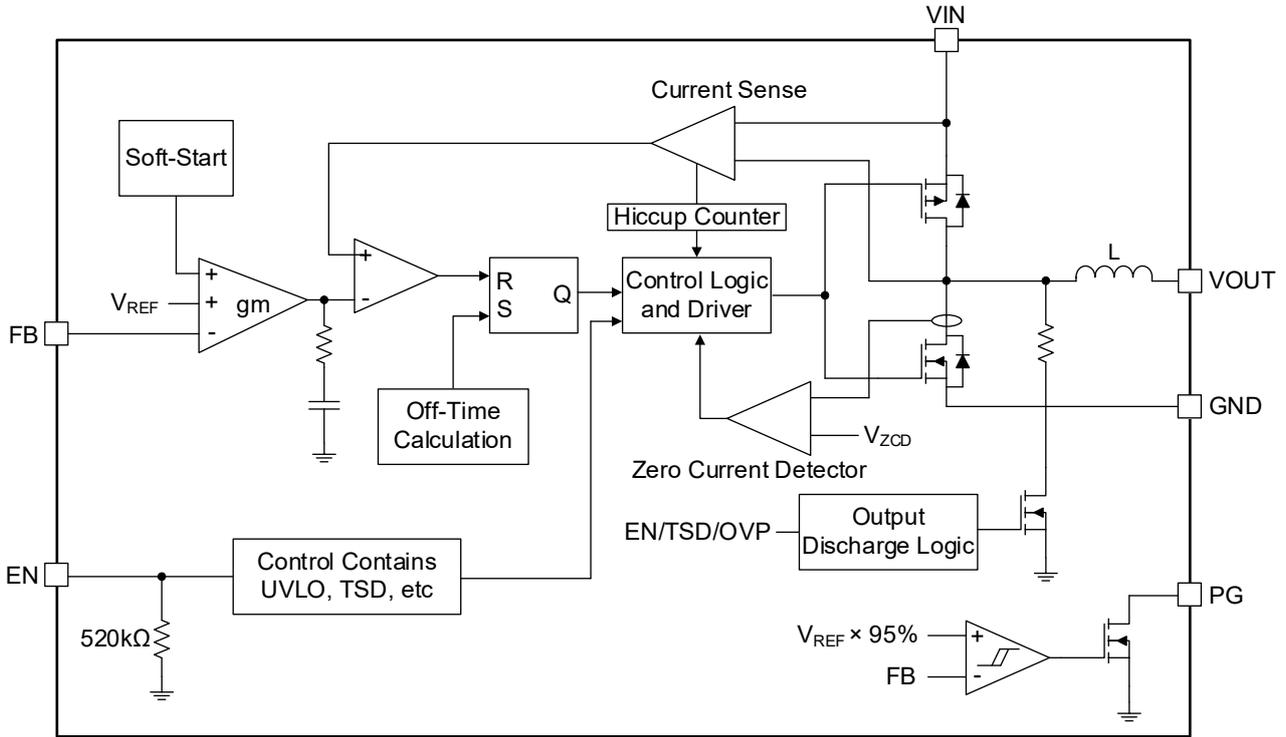
Figure 2. Block Diagram
