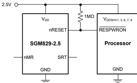
**Figure 6. SGM829 Typical Application circuit with a Microprocessor**
