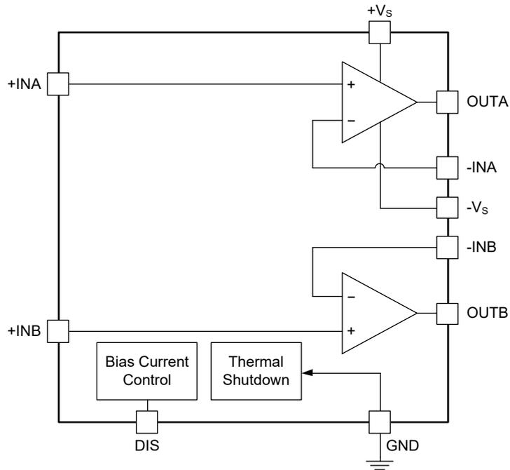
Figure 2. Block Diagram
