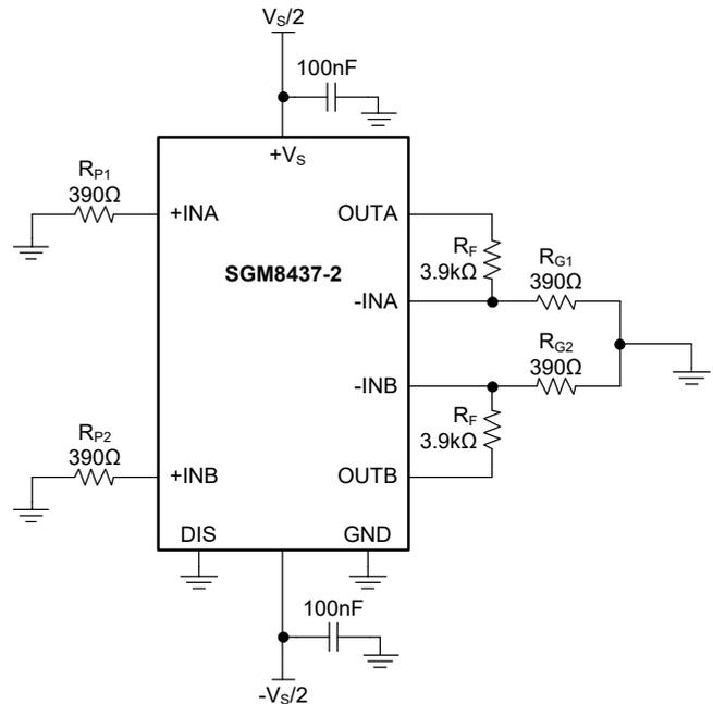
**Figure 3. Breakdown Supply Voltage Test Configuration**
